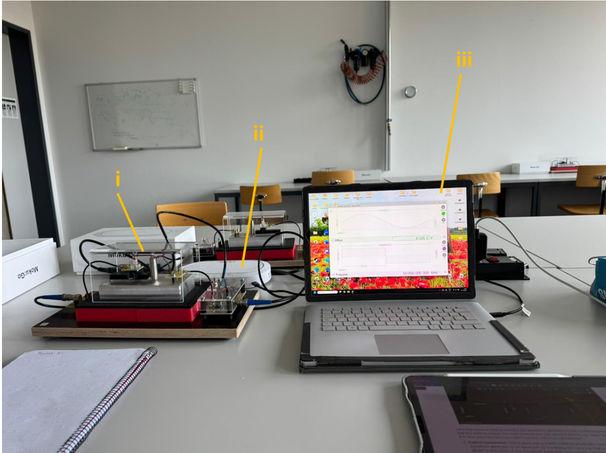
Figure 1: General set up for the experiment. On the left the cantilever and the piezo element are visible (i). In the background is the Moku:Go (ii) and on the right, a laptop with the Moku application (iii).
