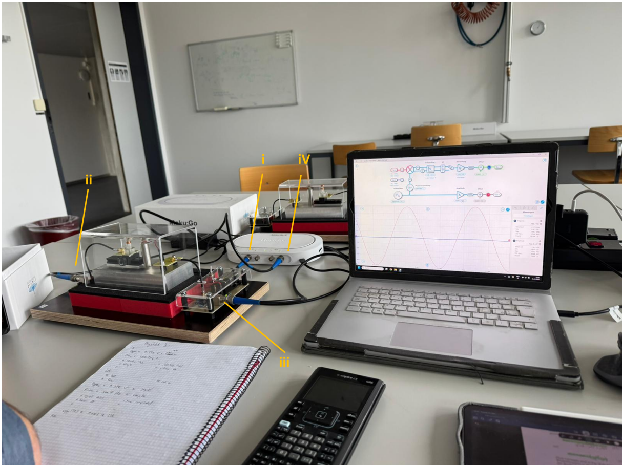
Figure 2: Set up for the third, fourth and fifth experiment. Moku:Go output 1 (i) is connected to the input of the cantilever(ii) and the output of the piezo element (iii) is connected with the input 2 of the Moku:Go (iv).
