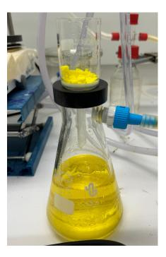
This solid was then dissolved in boiling hot ethanol for the recrystallization. The yellow solid dissolved and then the round bottom flask was left to cool down to room temperature. After that it was put into a ice bath to cool down further. The contents of the round bottom flask were put into a frit with a vacuum again and on the frit there remained a yellow solid, lumpy powder, this is the product 4-(4-nitrophenyl)morpholine.
