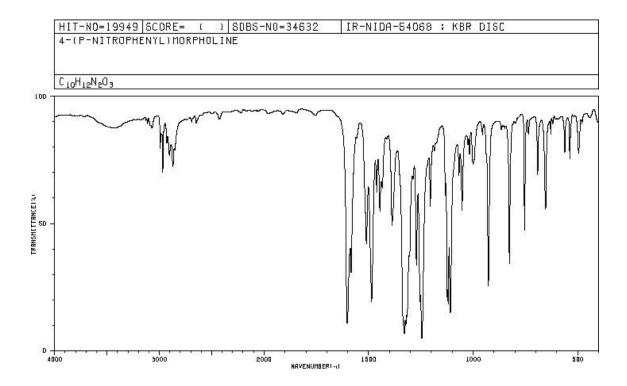
And this would be the measured infrared spectrum of the synthesized 4-(4-nitrophenyl) morpholine from the author.
