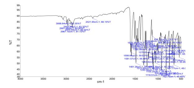
In the spectral analysis, the observed peaks mostly align with those documented in the literature, although they are weaker in intensity [3]. The wavelengths are accurate, but the absorption rates are lower, indicated by the T%, potentially due to the presence of impurities, variations in sample concentration, or the influence of the instrument's sensitivity and configuration.
