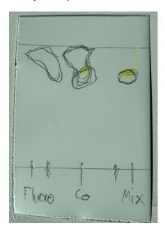
The educt 4-fluoronitrobenzene rose up higher than the product 4-(4-nitrophenyl)morpholine. The polarity of 4-fluoronitrobenzene may be higher than of the product, but there are also other factors in the rise of a TLC plate.
