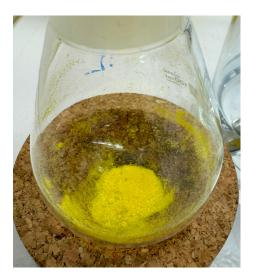
The weight of the product is 0.32 g. But the product still had some ethanol in it, that bumped up the weight. So the round bottom flask with the product was put into a rotarotary evaporator to remove the ethanol. After 20 minutes in the rotarotary evaporator the round bottom flask was removed and the weight of the product was measured again. The weight was 0.11 g (0.53 mmol, 0.11 equiv.), that would be a yield of around 10.57%.
