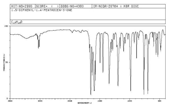
And this would be the measured infrared spectrum of the synthesized dibenzalacetone from the author.
