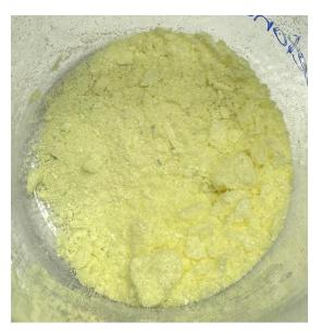
The resultant solid was filtered and washed with water. Recrystallization from ethanol yielded a yellow crystalline solid of (E,E)-Dibenzylideneacetone (1.373 g, 5.86 mmol, 0.51 equiv.) with a yield of about 51%.
