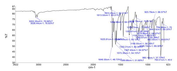
In the spectral analysis, the observed peaks align with those documented in the literature, although they are weaker in intensity [9]. The wavelengths are accurate, but the absorption rates are lower, indicated by the T%, potentially due to the presence of impurities, variations in sample concentration, or the influence of the instrument's sensitivity and configuration.
