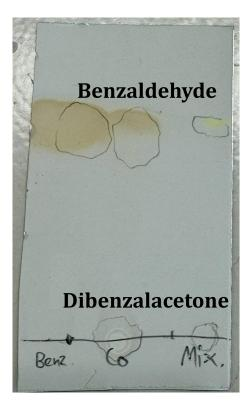
In this TLC, a silicate plate was used and there were three columns. The first column (Benz) had only one educt, the benzaldehyde. The second column (Co) had benzaldehyde and the yellow liquid mixture with the product dibenzalacetone on it. The third column (Mix) only had the yellow liquid mixture on it. The solvent consisted of 1 part n-Hexane and 1 part ethylacetate.
